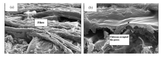
FIGURE 2. SEM micrograph show a comparison of surface morphology in cross sectional cut A4 printing paper (a) before and (b) after coating at 1000× magnification
